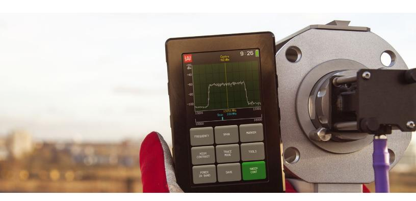
Link troubleshooting using Spectum Compact. SAF's Spectrum Compact can perform link troubleshooting from the ground level making it an exceptionally efficient tool for field engineers.
