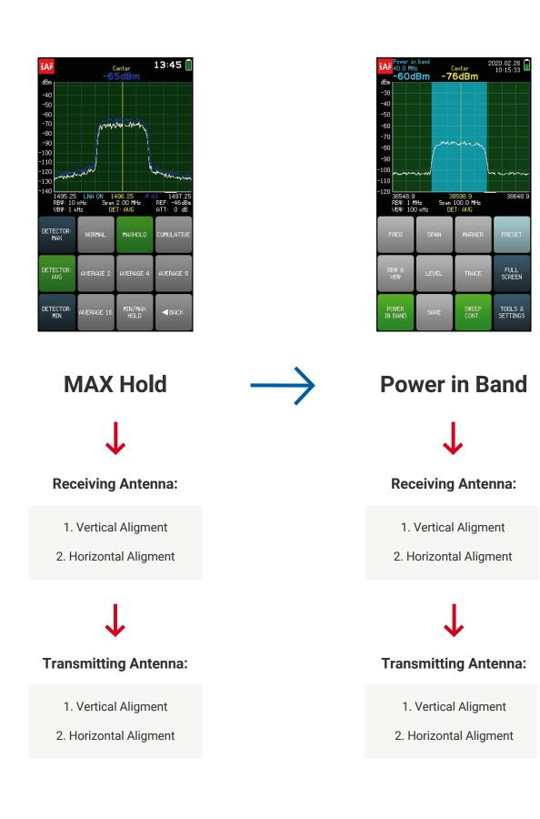
Fig. 9. Spectrum Compact functions aid in precise antenna alignment.
