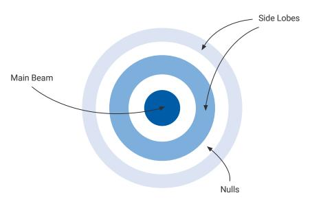
Fig. 7. Front view of the signal propagation
