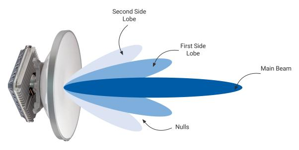
Fig. 6. Side view of the signal propagation
