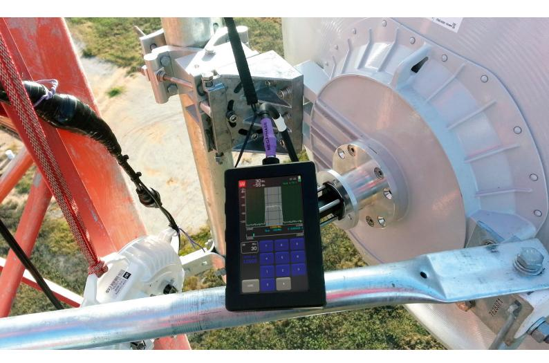
Fig. 3. Spectrum Compact connected to receiving antenna.
