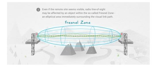
Fig. 5. Geometry of the Fresnel zone.
