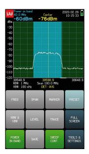
Fig. 11. Example of power in band measurement with Spectrum Compact. Light blue area indicates frequency span over which amplitude of signal is integrated.
