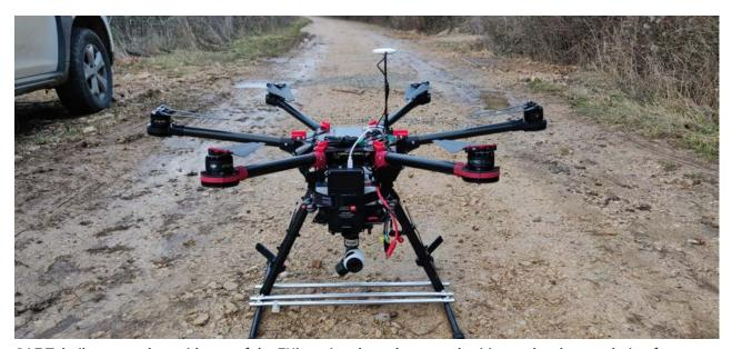
SAF Tehnika teamed up with one of the EU's national regulatory authorities to develop a solution for precise E-band link measurement and reporting using Spectrum Compact attached to a drone.
